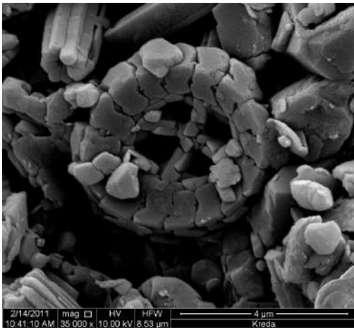
Fig. 5. Biomorphic structure of Cholm chalk writing in the image of scanning microscope
