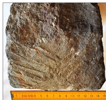
Figure 14. Example of hewing the side surface of a glauconitite block with a flat chisel with a blade width of 12-15 mm in two directions
