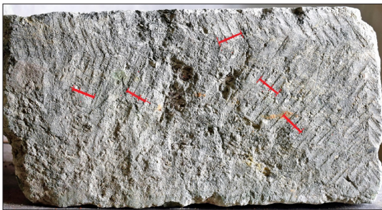
Figure 16. Surface of a glauconitite block with traces of cutting with a three-pronged flat mason's hammer
