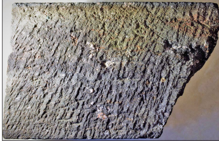
Figure 22. Example of final treatment of the front surface of a glauconitite block
