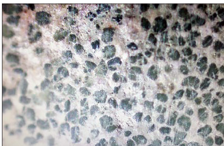
Figure 1. Surface of glauconite stone when magnified under a microscope
