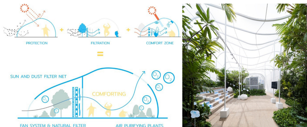
Figure 4. Air purification system using a greenhouse module, Thailand, 2021
