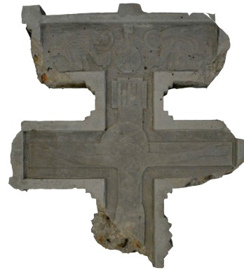
Figure 3. Memorial reinforced concrete cross from the Saint Assumption Univ Lavra museum's collections before conservation
