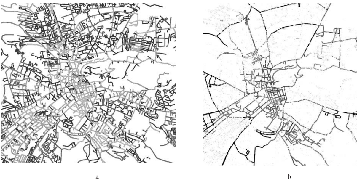
Fig. 2. Street network of the central part of Lviv city: a – a common network, b – identified as “prior spaces” according to the B. Hilliers method. Source: the author analysis
